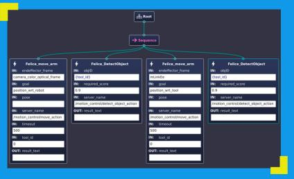
Behavior Trees (BTs) are increasingly favored for human-robot collaborative assembly tasks in industrial settings due to their hierarchical, modular structure [1]. BTs excel in managing complex assembly scenarios by breaking tasks into manageable sub-tasks, promoting fault tolerance, and ensuring real-time adaptability. Their organized architecture facilitates
