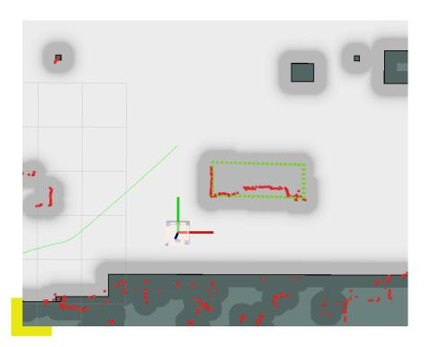
module does not return to correct operation, the platform will rotate to make it easier to find the current position, until a critical location error is reported.
